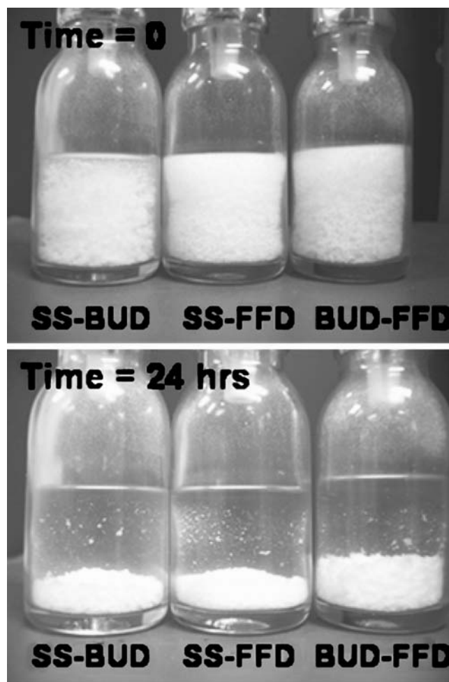
Fig. 8. Sedimentation of combination drug suspensions (SS-BUD = salbutamol sulphate in combination with budesonide; SS-FFD = salbutamol sulphate in combination with formoterol fumarate dihydrate and BUD-FFD = budesonide in combination with formoterol fumarate dihydrate). At T=0 , just after shaking, (top image) and after 24 h (bottom image).
